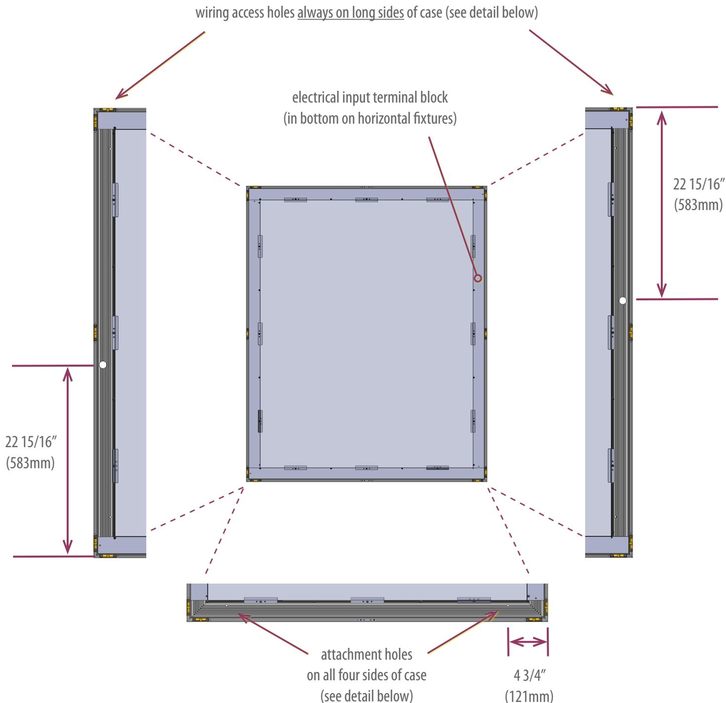
Wiring access holes — 1/2" trade size (7/8" [22.2mm] dia.), centered 1 1/6" (27mm) in from outside edge and 22 15/16" (583mm) in from end
