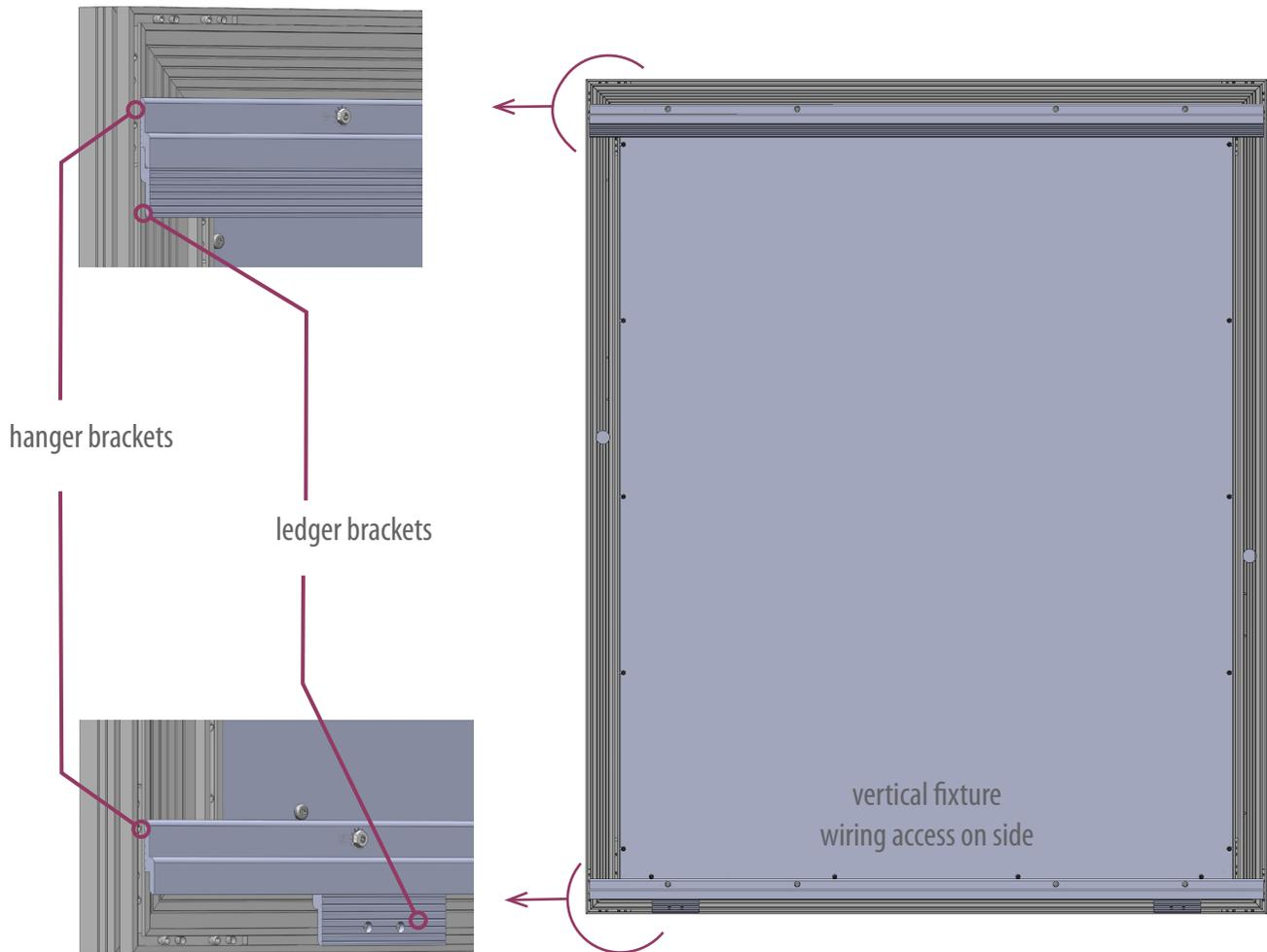
"Ledger" brackets are client-mounted on the wall:
