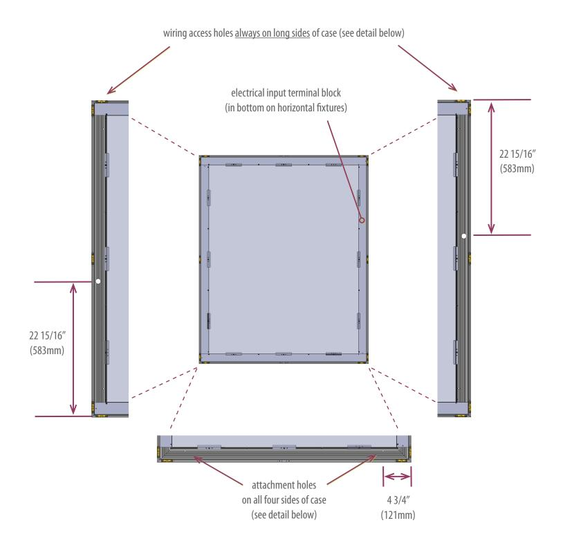
Wiring access holes — 1/2" trade size (7/8" [22.2mm] dia.), centered 1 1/6" (27mm) in from outside edge and 22 15/16" (583mm) in from end
